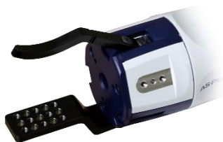
2-finger option mounting example
