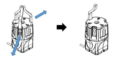
2. Fix the 2 fingers option with the screws and parallel pin.
